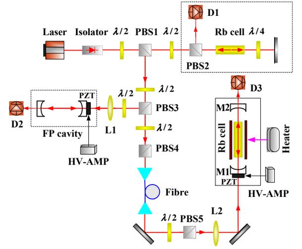
FIG. 2: (Color online). Schematic of the experimental setup of the coupled atoms-cavity system.  $\lambda/2$ : half-wave plate;  $D1$ ,  $D2$ ,  $D3$ : detectors; HV-AMP: high voltage amplifier; PZT: piezoelectric transducer; PBS: polarized beam splitter;  $L1$ ,  $L2$ : optical lens.
